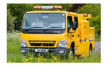
The measurements can be used to identify lengths of road that are at or below investigatory levels defined for particular road categories. A SCRIM machine survey in the UK can be undertaken at two different target test speeds 50 and 80 km/h.
