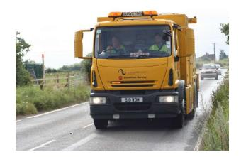
SCRIMTEX is a development of the SCRIM machine and supplements the wet road skidding resistance by measuring the surface macro-texture in front of the test wheel. This can be achieved in both wheeltracks of a double-sided SCRIM vehicle and provides, in conjunction with air and surface temperature, the ultimate requirement for the assessment of road surface condition monitoring for network surveys. Processing is undertaken using a suite of computer programs.
