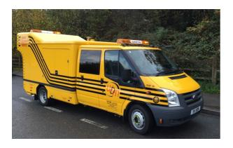
**Road Assessment Vehicle (RAV).** These vehicles provide measurements of the surface condition of a road, including cracking, to the SCANNER specification at normal road speed. The measurements monitor changes in the condition of networks and provide various key performance indicators helping clients prioritise maintenance.
