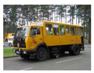
**UKPMS Coarse Visual Inspection (CVI) Surveys.** WDM<sup>®</sup> is a major provider of CVI surveys to local authorities and its large team of fully certified and experienced surveyors uses accredited software and vehicles specifically design to collect visual data. The WDM® solution includes digital mapping, data input via touch screen, real time processioning and defined collection rules and survey routes.
